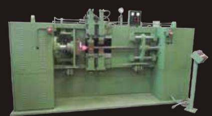
**METAL GATHERING MACHINE 250 KVA HORIZONTAL TYPE FOR SHAFTS**
