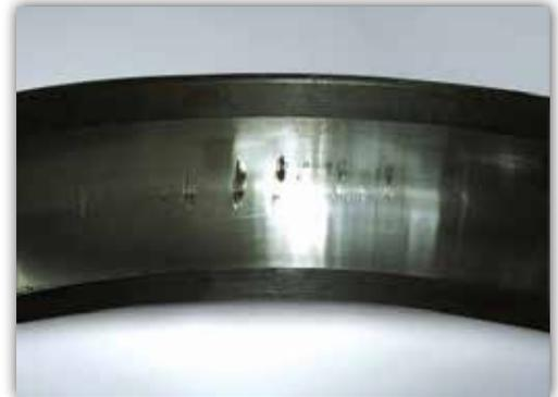
even with low currents, can lead to electrical damage.
