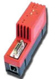
conversion can be either slave to slave or slave to master. As a master, netTAP 50 provides full master functionality to one slave device only. ■
