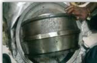
6. **Corrosion.** Moisture, acid, low-quality or broken-down grease, poor wrappings and condensation from excessive temperature reversals can cause corrosion.
