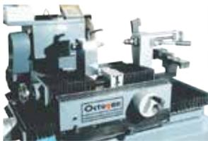
PRECISION RECESS GRINDING MACHINE
