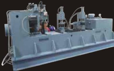
**METAL GATHERING MACHINE 100 KVA HORIZONTAL TYPE FOR TORSION BARS & STABILIZER BARS**
