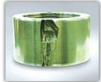
8. **Fatigue (Spalling).**
