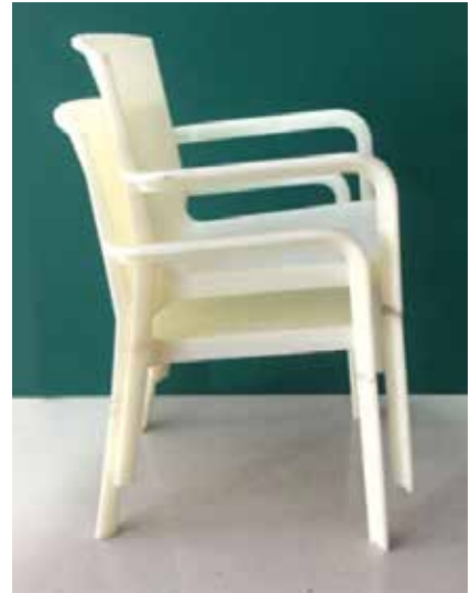
These stacking monobloc chair models were 3D printed in ABS material to check the viability of the design.
