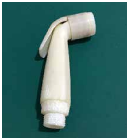
A prototype water spray nozzle 3D Printed in ABS material to validate the nozzle size and flow capacity to withstand the speed of water.
