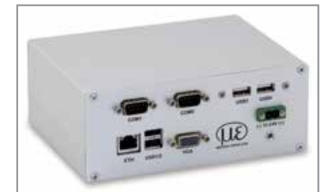
thermoIMAGER TIM NetPCQ PC solution for thermal imager applications
