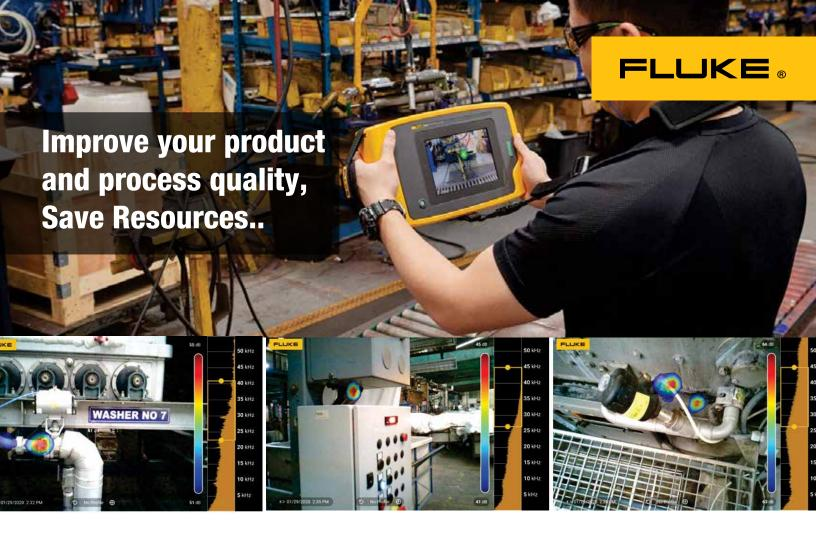
Save time and resources with Fluke Acoustic Imager! Find the leaks instantly and improve your pneumatic system's performance.
